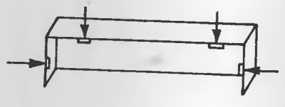
FIGURE A FIGURE B FIGURE C NOTE: THE CABINET SECTIONS ARE HELD TOGETHER WITH SNAP TABS SHOWN BY ARROWS. SEE FIGURES A AND C.
